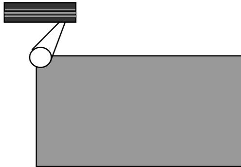
Heading the first corner on the left backside of stage with the beam (To be sure to get the same corner points for all the scans, the corners should be marked on stage with white tape crosses.)
